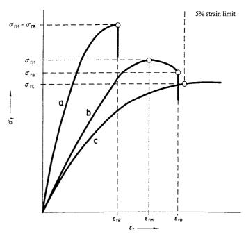
NOTE—Curve a: Specimen that breaks before yielding. Curve b: Specimen that yields and then breaks before the 5 % strain limit.
