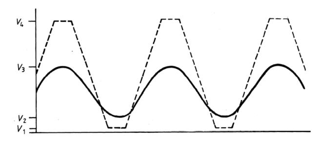
Figure 2 — Calibration waveforms — AC method
