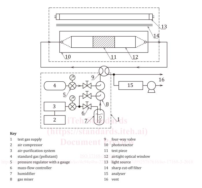
Figure 1 — A schematic of the testing equipment
