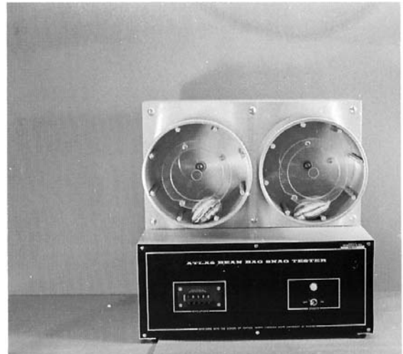
FIG. 4 The Bean Bag Snag Tester With Two Test Chambers
