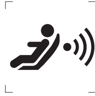
Figure 1 — Symbol for automatic child seat presence and orientation detection system (CPOD), ISO 7000-2960
