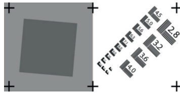
Figure 5 — Example of MTF measurement features
