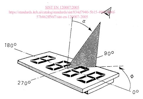
Viewing angles  $\alpha$  and  $\tilde{\Phi}$  are defined according to the above figure
