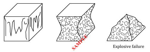
NOTE All four exposed faces are cracked approximately equally, generally with little damage to faces in contact with the platens.
