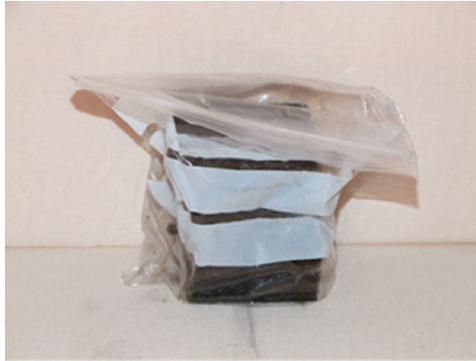
Figure 2 — Ignition source (exemplarily)
