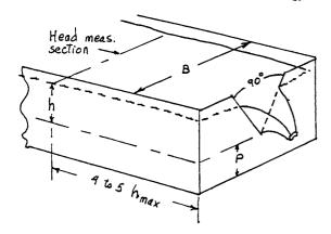
Limitations on geometry:<sup>B</sup>  $h/P \le 1.2$   $h/B \le 0.4$   $P \ge 0.3$  ft (0.1 m)  $B \ge 2$  ft (0.6 m) 0.15 ft (0.05 m)  $\le h \le 2$  ft (0.6 m)
