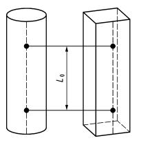
a) Measurement points in a line parallel to principal axis
