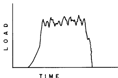
FIG. 1 Load-Time Chart for Low-Extensible Film
