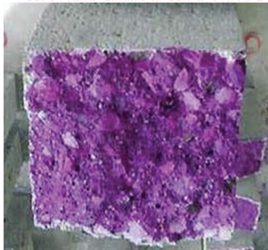
Figure 1 — Phenolphthalein indicator as used on a freshly exposed surface of good quality concrete
