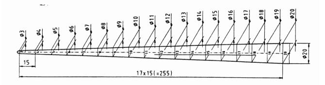
Figure 1: Gauge for determining knotability K
