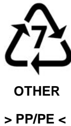
Figure 2 — Marking of polypropylene-polyethylene copolymer battery components
