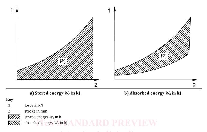
Figure 1 — Force stroke diagram for stored and absorbed energy
