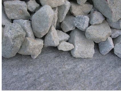
Figure 1 — Drainage aggregate in contact with protection geotextile
