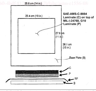
C = SAE-AMS-C-9084 Laminate, 20 nested plies of SAE-AMS-C-9084 Type 7781 glass cloth impregnated with test epoxy resin system
