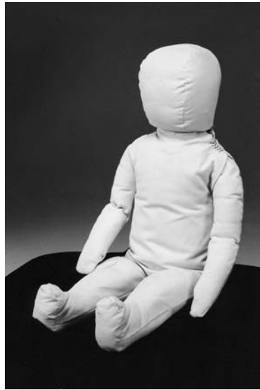
FIG. 1 CAMI Dummy, Mark II
