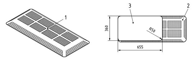
b) Fail, more than 50 % of the projected open cross section is covered (dome shaped)
