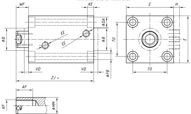
NOTE Pilot extension is optional. The dimensions *B* and *VD* should be used if pilot extensions are needed.
