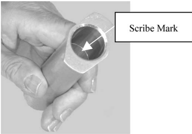
FIG. 4 Syringe Barrel with Scribe Mark
