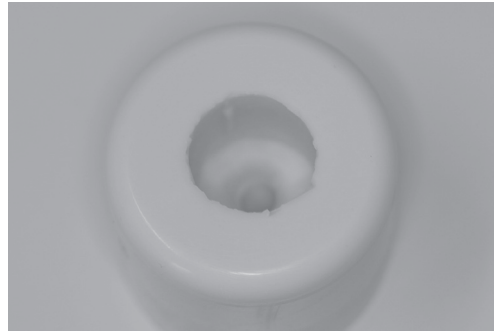
Figure 3 — Silicone mould for production of the test specimens
