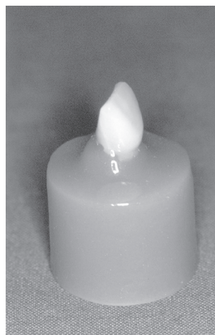
Figure 2 — Test specimen made from modelling wax and polymer tooth
