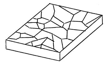
fin-fine feather-edge protrusion from the surface (Syn. flash).
