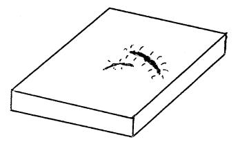
crazing—the cracking that occurs in fired glazes or other ceramic coatings as a result of tensile stresses, may also occur in the
