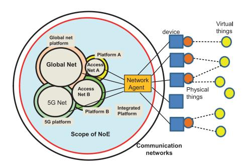
Figure 1 — Conceptual model of NoE and its scope from the network handover point of view
