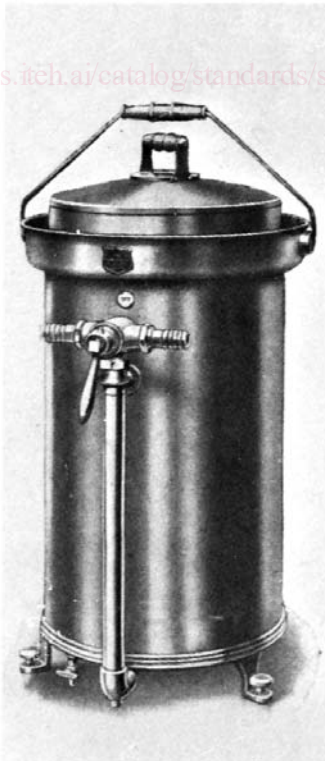
FIG. 1 Stillman-Type Portable Cubic-Foot Standard
