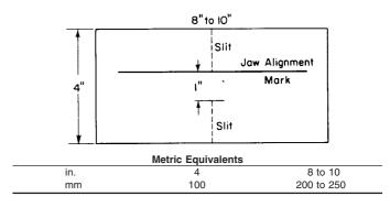
FIG. 2 Illustration of Modified Grab Test Specimens
