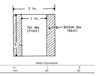
FIG. 1 Schematic Illustration of Jaw Faces for Modified Grab Test
