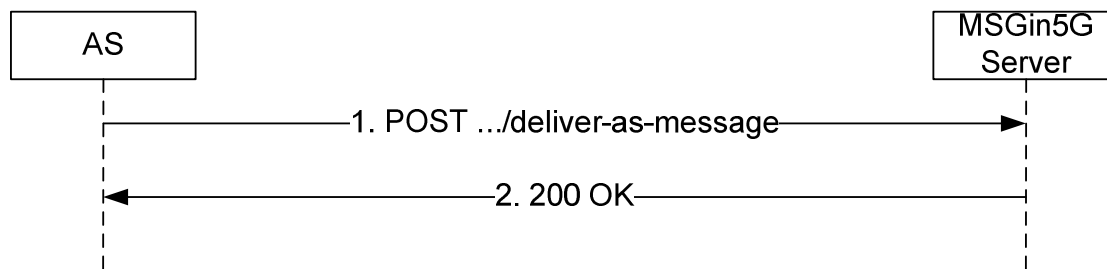
Figure 5.3.2.2.2-1: AS Originating MSGin5G Message Delivery
