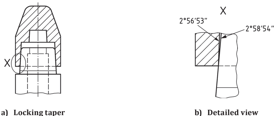
Figure 1 — Principle of a locking taper
