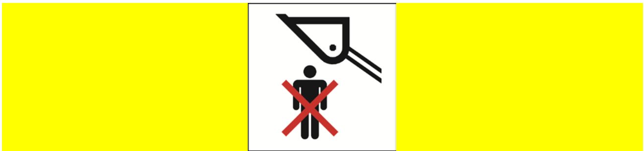
Figure B.17 — Do not stand under bucket
