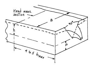
Limitations on geometry:  $^B$   $h/P \le 1.2$   $h/B \le 0.4$   $P \ge 0.3$  ft (0.1 m)  $B \ge 2$  ft (0.6 m) 0.15 ft (0.05 m)  $\le h \le 2$  ft (0.6 m)
