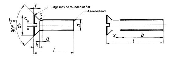
Shank diameter is approximately equal to pitch diameter or equal to major thread diameter permissible
