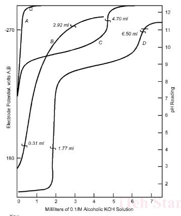
Key: Curve A—Blank on 125 mL of titration solvent.
