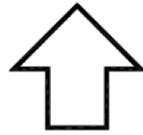
Figure 1 — Pictogram ISO 7000 - 1861 Indication for vertical alignment
