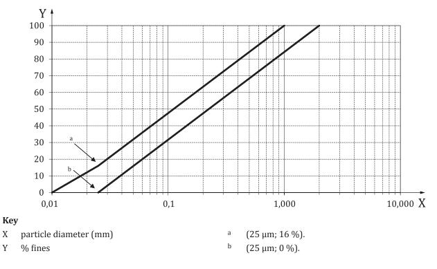
Figure 4 — Required zone of the cumulative percentage of size distribution of the granular material used
