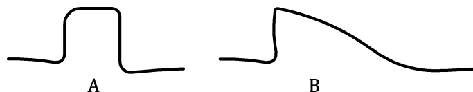
Figure 2 — Example of a good (A) and a bad (B) carbon disulfide solvent peak shape, obtained under cryogenic conditions
