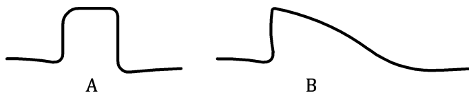
Figure 2 — Example of a good (A) and a bad (B) carbon disulfide solvent peak shape, obtained under cryogenic conditions
