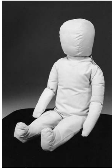
FIG. 1 CAMI Dummy, Mark II
