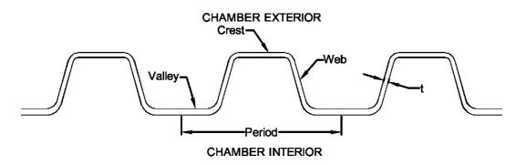
Note—The corrugation profile shown in this standard is intended only as a general illustration. Any corrugation pattern is permitted, as long as it meets all the specified test requirements of this standard.
