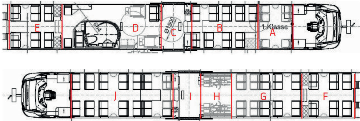
Figure 1 — Example of a possible choice dividing a DMU into 10 areas A to J
