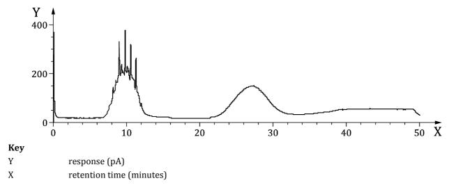
Figure 2 — Typical chromatogram of binary gravimetric blend distillate
