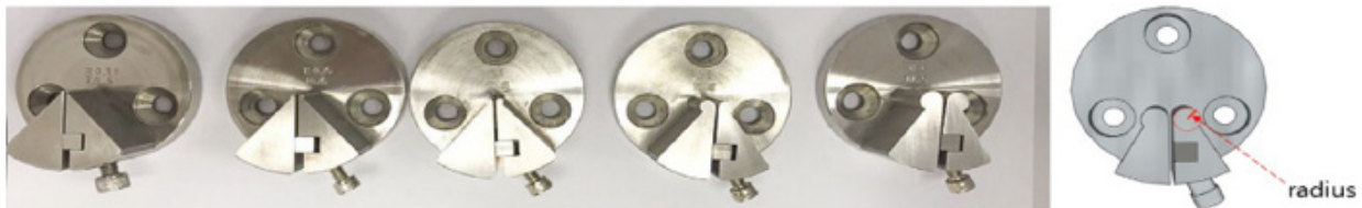
224 Figure 5 – MIT folding jigs (from the left, folding radius r is 1,0 mm, 2,0 mm, 3,0 mm, 225 4,0 mm, 5,0 mm and 10,0 mm)
