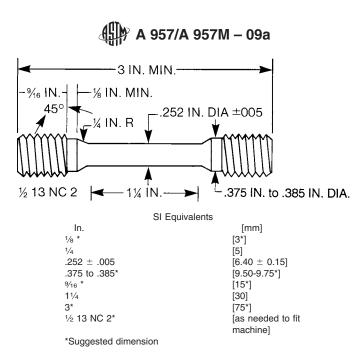
FIG. 1 Design and Dimensions of the ICI Test Bar
