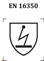
Figure 2 — Example of marking for electrostatic properties of gloves according to EN 16350 and ISO 7000-2415
