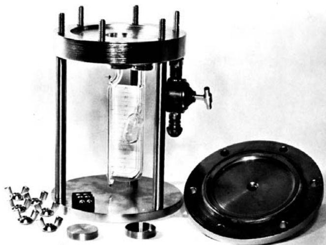
FIG. 1 Manometric Gas Transmission Cell
