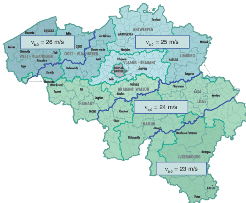
Figure 4/BE.1 – Basic wind velocities V_{b,0} according to NBN EN 1991-1-4 ANB
