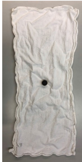
Figure 1 — Placing the data logger in the centre of a towel according to step 1
