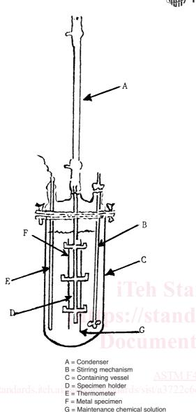
Note 1—This is one form that the equipment can take, and is not mandatory. Any array meeting the requirements of 4.2-4.5 is acceptable. FIG. 1 Test Apparatus
