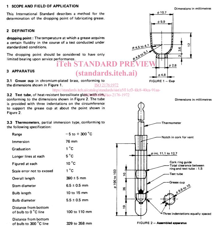
**3.4** Accessories: An oil bath consisting of a 400 ml beaker and suitable oil, a ring stand and ring for support of the oil bath, clamps for thermometers, two corks as illustrated in Figure 2, a polished metal rod 1.2 to 1.6 mm in diameter and 150 mm in length and suitable means for heating and stirring the oil bath. Heating shall preferably be effected by an immersed electrical-resistance heater regulated by voltage control.
