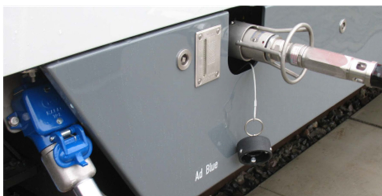
Figure 1 — Typical installation of AUS 32 coupling and electrical connector
